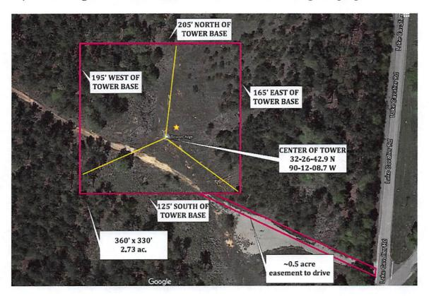
The center of the tower would be at approximately 32-26-43 N, 90-12-09 W (NAD 27), with the guy wires shown above to scale.
